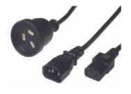
female connector. Length is 600mm overall, comprising 2 x 220mm IEC sections and a single 220mm section from the mains socket to the Y-junction. Electrical Safety Authority Approved.
